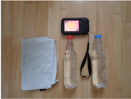
Fig. 12. Experiment preparation aids – two PET bottles filled with water of the same temperature, thermovision camera and a towel.
